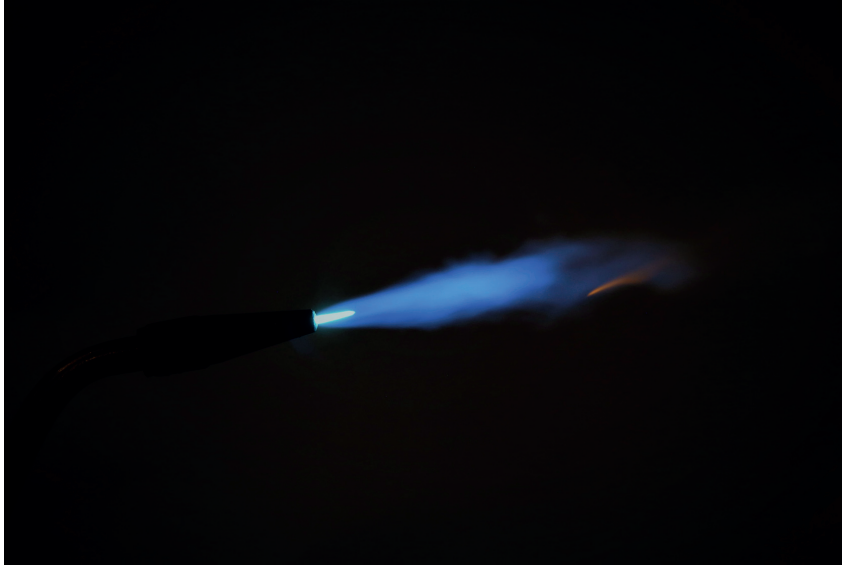
Figuur 6 Reducerende of neutrale vlam
